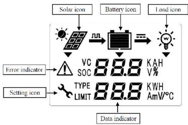
The two LED indicators above the LCD show that battery is charging, and a red indicates error conditions. The LCD has two different brightness levels. After any button is pressed the display will be in high brightness and backlight. To save power, the backlight automatically turns off after 30 seconds.
