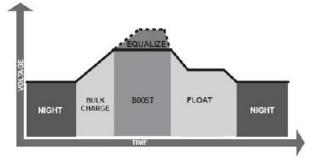
heating and excessive battery gassing. The Boost stage remains 120 minutes and then goes to Float Charge. Every time when the controller is powered on, if it detects neither over discharged nor overvoltage, the charging will enter into boost charging stage.
